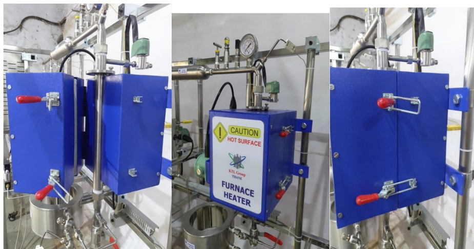
Figure 27: Reactor and Furnace Assembly
